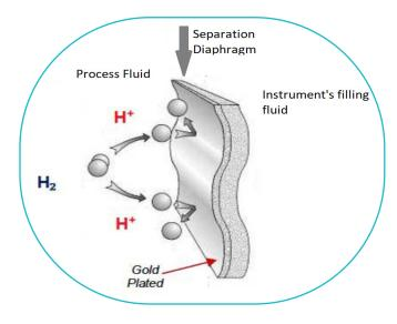
On mechanical products such as Bourdon tube pressure gauges or Bourdon diaphragm, or bellows actuated pressure switches, this effect is not seen.
