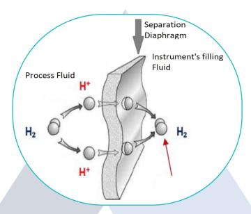
The H2 molecules will then be trapped inside the fill fluid of the transmitter because they are once again too large to pass back through the isolation diaphragm.
