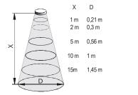
Diameters corresponding to 5° beam angle.
