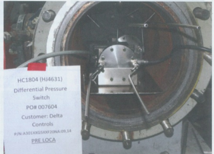
Left: Delta Switches being seismically tested to RCC-E requirements at the SOPEMEA test facility in France.
