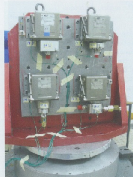
Delta Switches being seismically tested to RCC-E requirements at the SOPEMEA test facility in France.
