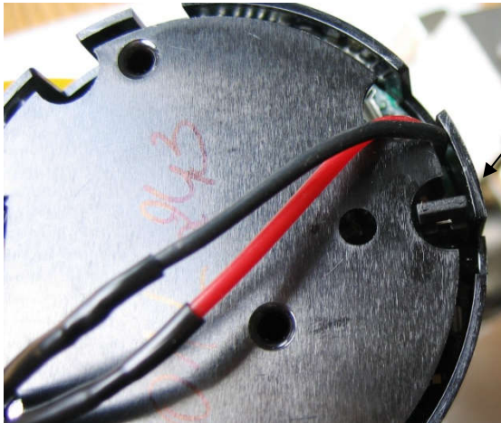
Fig. 5. Back lighting jumper view at transmitter electric board (unit display back side) (for version Exd).
